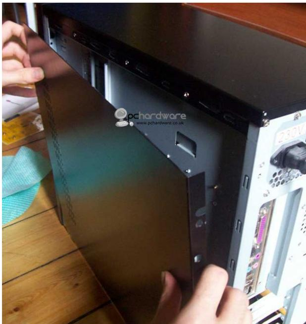
2. Wearing an anti-static wristband is desirable whenever working with sensitive electrical equipment. Keeping one hand on a metal part of the case will have the same effect, though you may need both hands when installing certain items of hardware.
